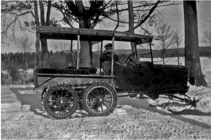
Guy Crouse used this Model T "snowmobile" for the Stage, carrying mail, passengers, and purchases from the stores.
