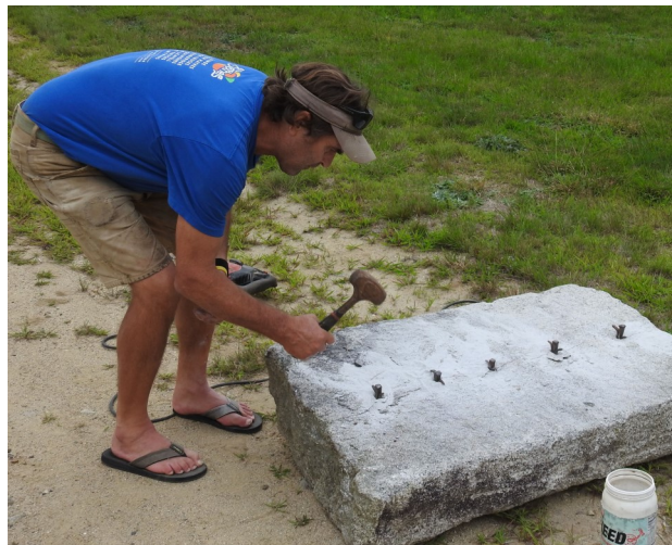
Harrison "Micky" Hoyt IV used feathers and wedges to split a piece of granite to make a raised flower bed at our school-house. One final piece is ready to be split during the Town Picnic
